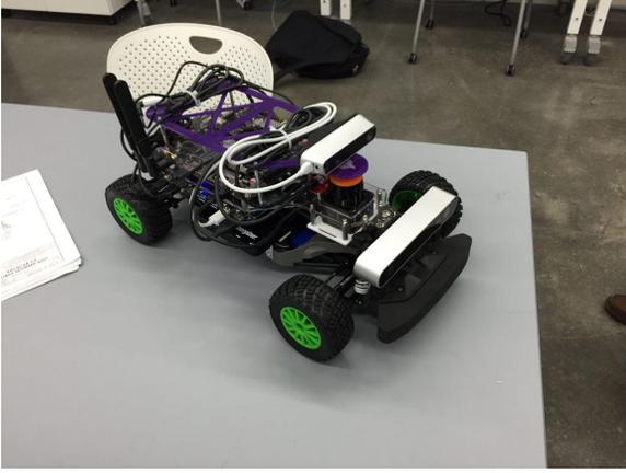
Fig. 1. Remote-controlled car used in the project. The shell was detached and sensors and an embedded system were placed on it. The ZED camera is mounted on the front of the car.
